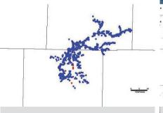
Cloud lightning flash detected in the Dallas-Fort Worth area of Texas, USA. The blue dots show VHF cloud lightning mapping and the red dots show VLF/LF cloud lightning detection. The total length of this cloud flash as shown by VHF cloud lightning mapping is 50km
