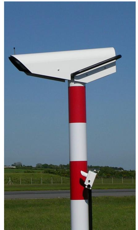
LM21 measures the ambient light level or background luminance in RVR applications. In the picture, LM21 is installed on Vaisala Transmissometer LT31.
