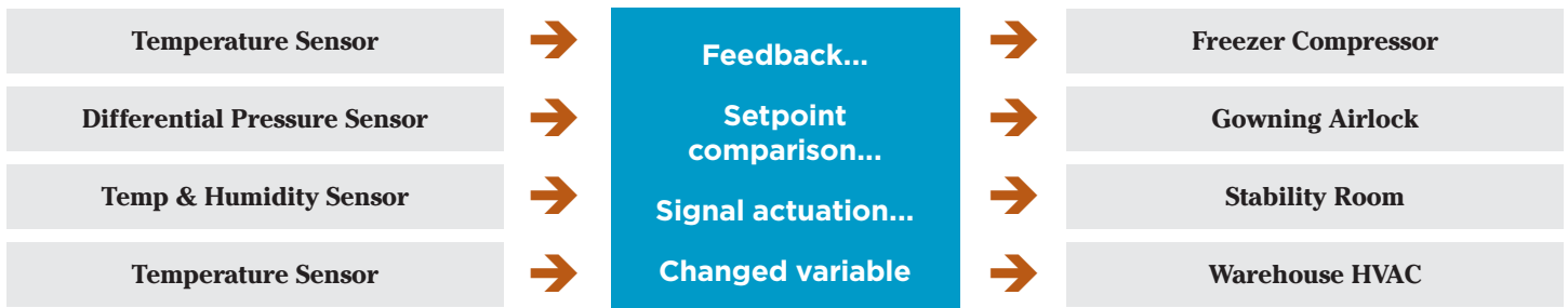
Control system with central points of electronics failure.
