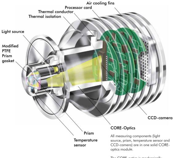
The CORE-optics is mechanically isolated from the influence of external forces and vibrations. The CORE-optics contains no mechanical adjustments.
