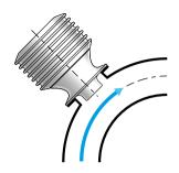
2.5 inch Sanitary clamp and flow cell
