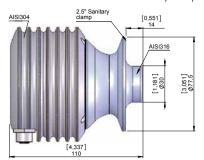
EFC Flow cell, 2.5 inch line diam.
