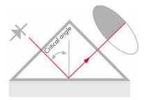
A CCD-camera detects the optical image. The image is transformed point-by-point into a digital signal. Digital signal processing is used to locate the exact shadow line position and to determine the refactive index  $\rm n_{\rm p}$ .
