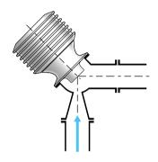
2.5 inch Sanitary clamp and flow cell
