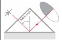
A digital CCD-camera detects the optical image and the shadow line. The camera transforms the optical image point-by-point to an electrical signal. The exact shadow line position is located and converted to a reading in refractive index.
