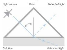
All rays coming to the surface below a certain angle, are totally reflected. The light coming to the surface at a higher angle is refracted into the process solution.
