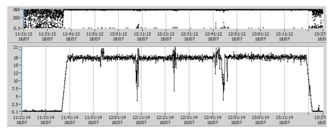
**Figure 8**. Measurement data from the UUT during the test period. Upper graph is wind direction and lower is wind speed. Changes on wind speed value were due to the ice thickness measurements.
