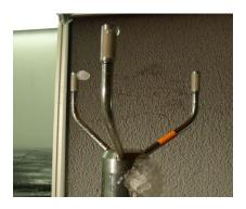
**Figure 3**. UUT after icing period. Ice layer on non-heated structure was 27 mm, while sensor tube has ice of 24 mm.
