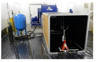
**Figure 2**. Test set-up includes water tank (blue), radial blower, air channel, water spraying nozzles, and UUT inside climate cabinet.
