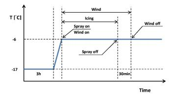
**Figure 1**. Test profile.  $1^{st}$  phase is cold soak period,  $2^{nd}$  phase is icing period with icing and wind,  $3^{rd}$  phase is wind period.
