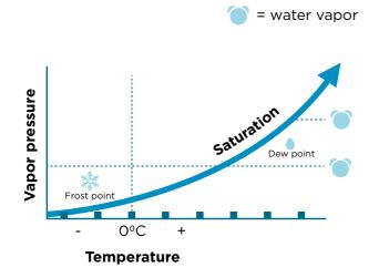
It's important to know which output parameter to use in order to get the most accurate process. If we look at a compressed air system, the frost point temperature is often around -40 °C (-40 °F). This equals about -44 °C (-47 °F) in dew point temperature. With these example values wrong parameter causes about 4 °C (7 °F) error.
