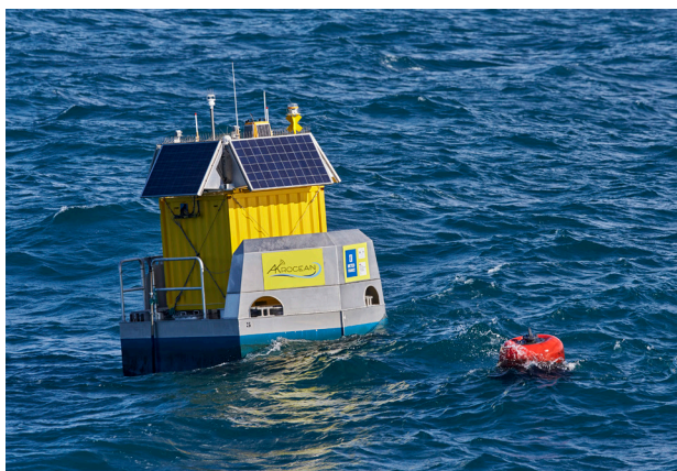
WindCube Offshore mounted on a buoy. See how AKROCEAN is enabling new offshore development in France.
