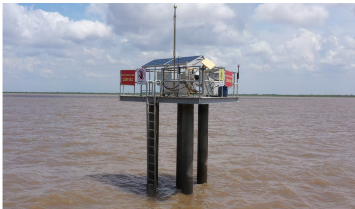
WindCube Offshore on a fixed offshore platform installation. See how Mainstream Renewable Power is conducting more accurate offshore WRA campaigns in Asia.
