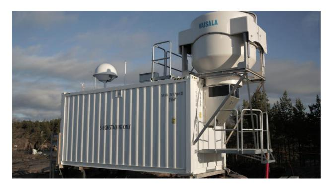
An automatic sounding system makes the sounding process efficient and reliable.
