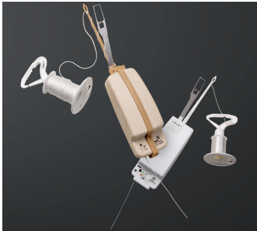
Figure 2. RS41 E-model with BioCover and BioTwine (left) and standard RS41 with EPS cover and non-biodegradable string (right).
