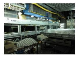
**Figure 1.** Snowing wind tunnel set-up. Fresh snow is fed to snowfall device from where is falls down to the wind tunnel, where the unit under test is located.
