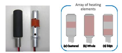
**Figure 5.** On left, the dummy scale model of a transducer stack had a wire heater embedded to a rubber. On right, the heating variation options of the dummy transducer stack were "centered", "whole", and "edge".
