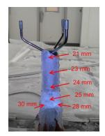
**Figure 6.** New sensor design was operative throughout the test period with the freezing rain test profile (Table 3). In this test, the body heating was inactivated.
