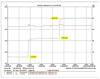
A typical 3-point data logger calibration cycle.
